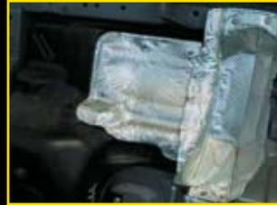
Multiple layer fuel tank heat shields
